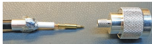
Figure 6 — The center pin being fitted.
