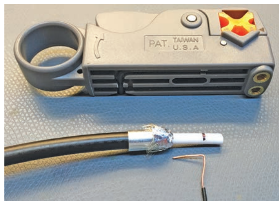
Figure 5 — The measured amount of dielectric is marked and then removed.
