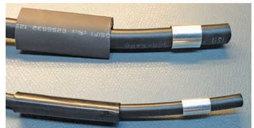
Figure 2 — Start with a square cut across the cable end and slide on the ferrule and a piece of heat-shrink tubing.
