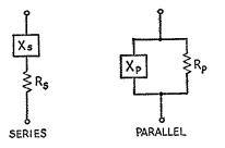
Fig. 1 — Series and parallel circuits containing resistance and reactance. By proper choice of constants, the two circuits will behave identically; i.e., the current and phase angle will be the same in both for the same impressed voltage.
