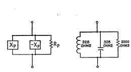
Fig. 4 — Reactance cancellation in the equivalent parallel circuit.
