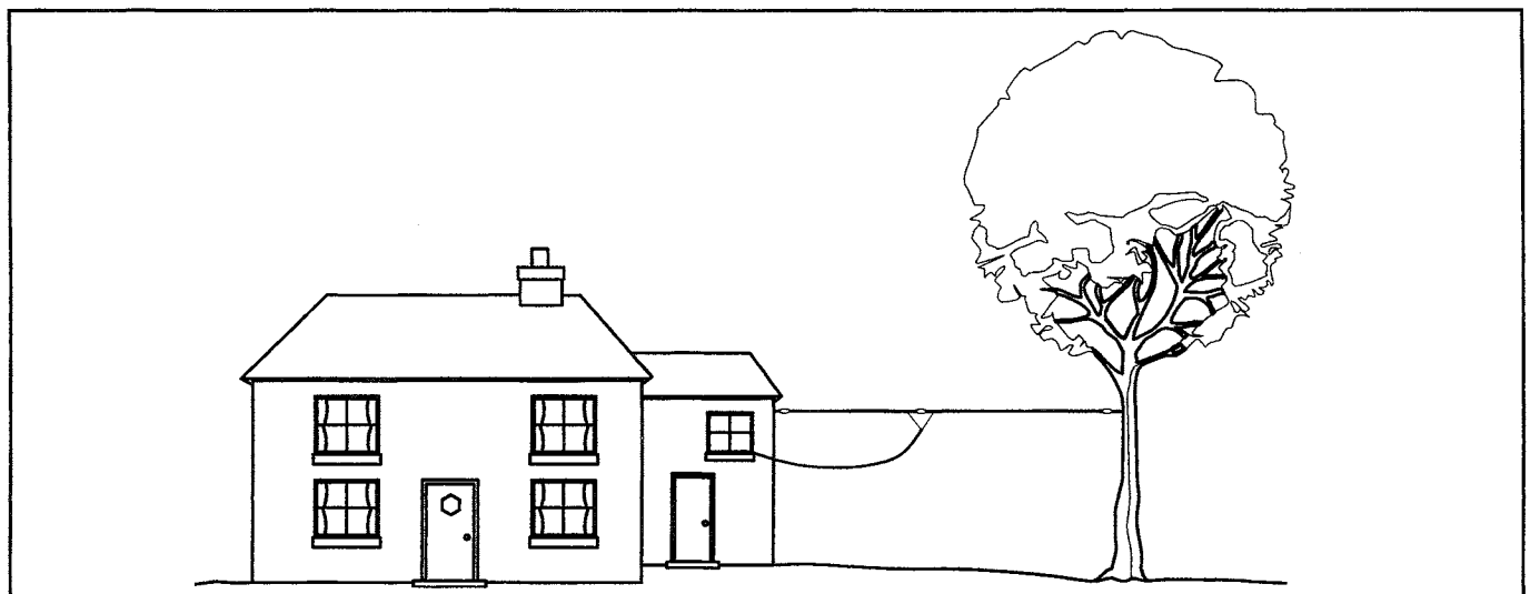
Figure 5.19—This feed line is very asymmetrical with respect to the antenna. This configuration could result in excessive feed line radiation—possibly a problem for the station operator or persons located near the feed line.
