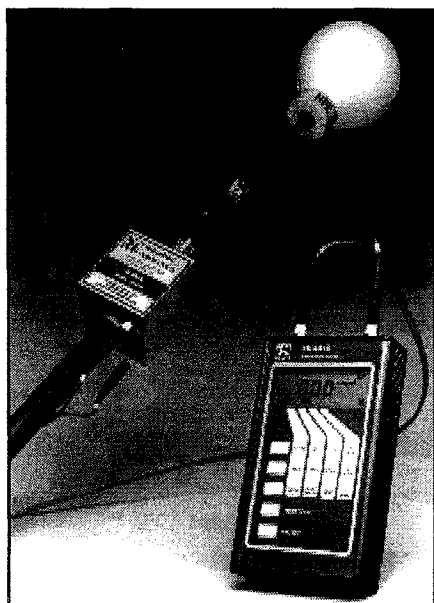
Figure 5.11—This calibrated field-strength meter and probes can be used to make measurements of the fields near a radio transmitter. (Photo courtesy of Holaday Industries, Inc.)
