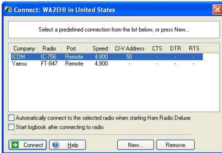
**Figure 9 - Connect Dialog Box with previously set up radios**
