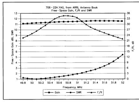
Figure 1—Graph of gain, F/R (front-to-rear ratio) and SWR over the 49.8 to 52.0-MHz range for 706-22H Yagi from *The ARRL Antenna Book*. The gain peaks at 51.6 MHz; the F/R peaks at 50.7 MHz. The matching network has been adjusted for a 1:1 SWR at 50.1 MHz.
