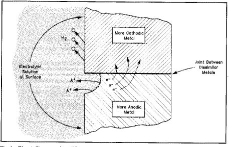
Fig 1—Bimetallic corrosion. When two dissimilar metals are joined in the presence of an electrolyte, the more anodic metal will corrode by releasing positive ions (A<sup>+</sup>). This frees electrons (e<sup>-</sup>) that move across the junction, forming hydrogen bubbles (H<sub>2</sub>) at the cathode. This is the same reaction that batteries use, except the electrons flow through a circuit.
