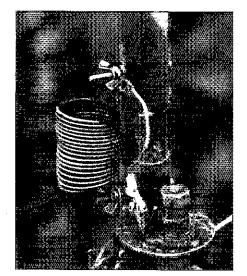
After assembly, this section of an antenna was painted. I used a brightly colored paint; in this case, red. Painting is especially useful where plastic tape is difficult to apply, or where an impracticably large amount of tape would be needed. When you need to disassemble a joint for cleaning, the bright color makes it easier to see if you've removed all the paint. (photo by the author)
