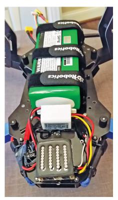
A drone with an EPM installed (the EPM is the square piece at the bottom of the photo).
