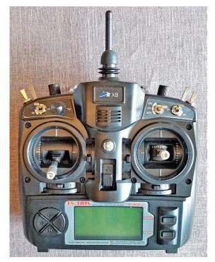
A drone controller with a twist knob potentiometer at the upper left that controls the EPM (similar to a camera gimbal control).
