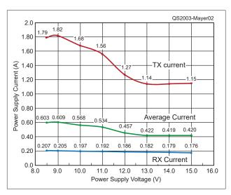
**Figure 2** — Power supply current versus voltage for the KX3. Other QRP radios have very different current versus voltage behavior.
