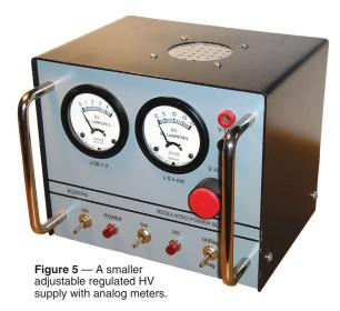
When set to any voltage between 160 V and 260 V, it holds that voltage under loads up to about 50 mA. Higher currents exceed the transformer capacity and the output voltage falls. Voltages up to 300 V can be set, but with less available current. The filament current supply can adequately support multiple-tube circuits.
