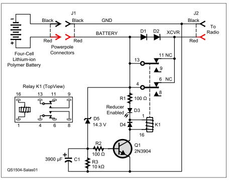
Figure 1 — Schematic diagram of the voltage reducer. Mouser (www.mouser.com) part numbers in parentheses.
