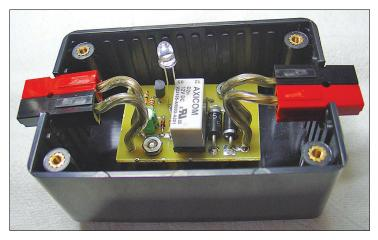
**Figure 4** — The voltage reducer mounted in a Hammond plastic box with Powerpole connectors slid into slots made with an inexpensive nibbling tool. The Reducer Enabled LED stands above the PC board to just poke through a hole in the box's top cover.
