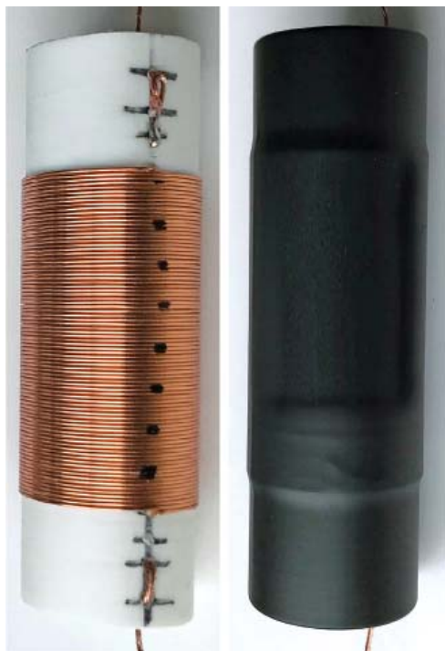
▲ Figure 2 — On the left, the loading coil is shown uncovered, and the right image shows it covered with heat shrink.
