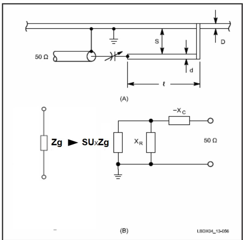
Fig 13-56—Layout and electrical equivalent of the Gamma match where SU is the step-up ratio and  $X_R$  is the inductive reactance from the gamma rod transmission line.
