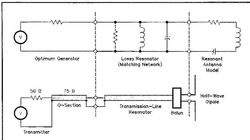
Fig A—Lossy broadband-matching-network equivalent circuit (top), and corresponding simple broadband antenna system elements (bottom).
