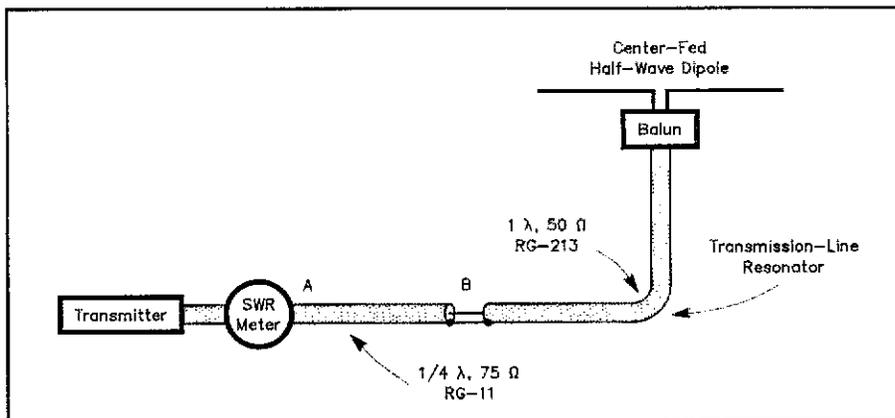
Fig 1—One form of the simple broadband antenna system. It resembles a conventional dipole except for the 1/4-wavelength, 75-Ω segment. Points A and B are discussed in the text.
